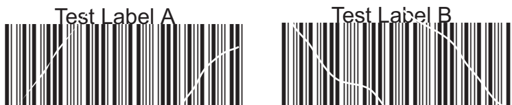
Low Quality Printouts Caused by Ribbon Wrinkling
