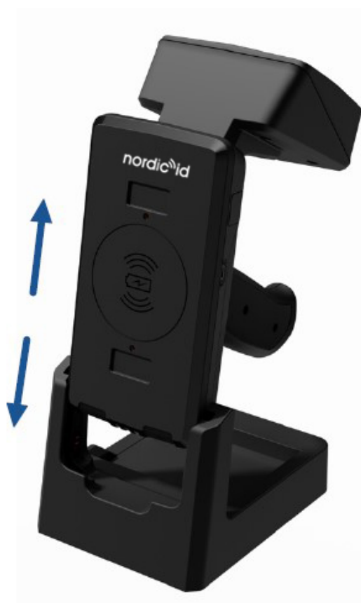
Picture 4 Charging of the Nordic ID EXA51e via cradle
