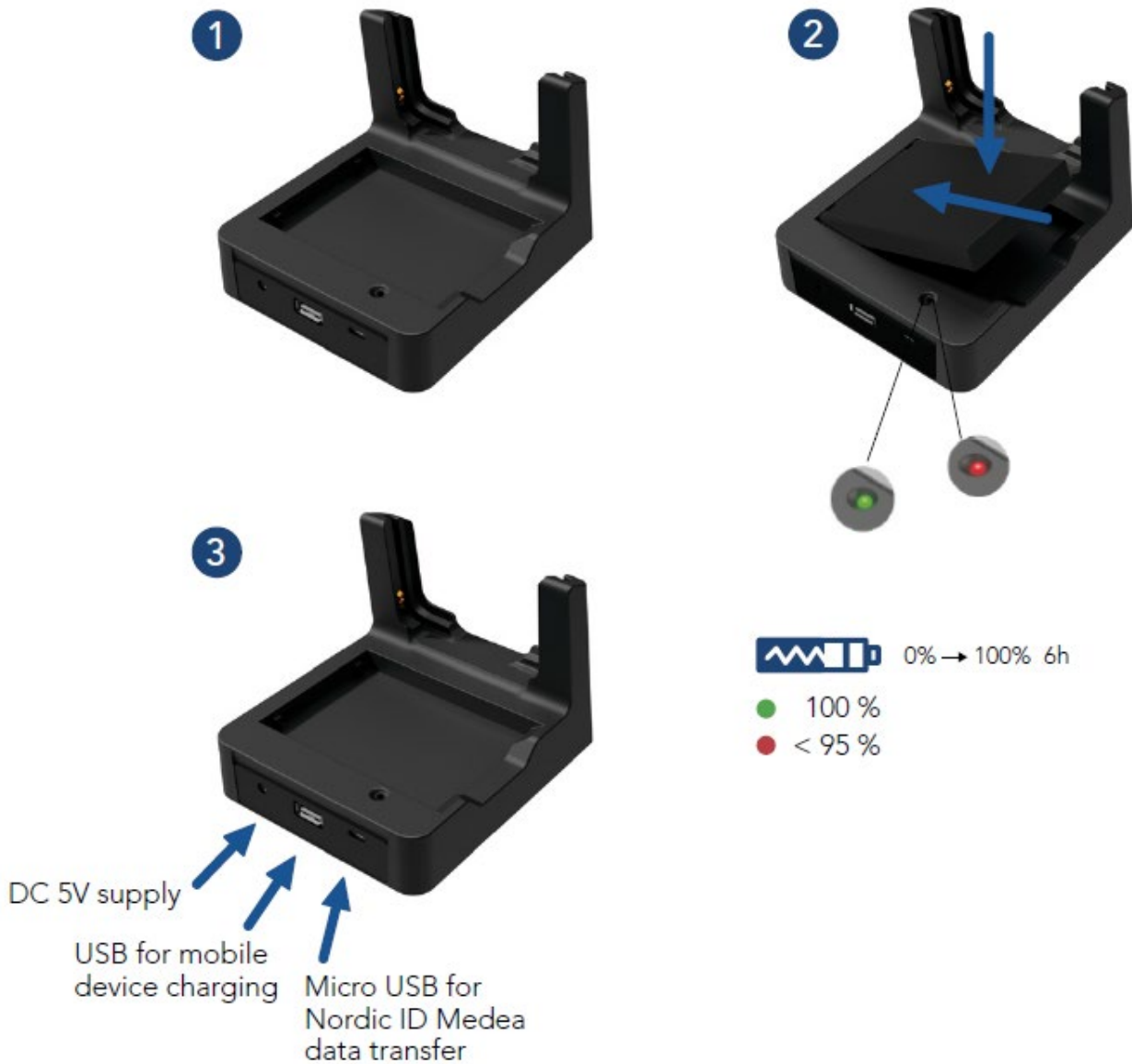
Picture 8 Battery charging in cradle
